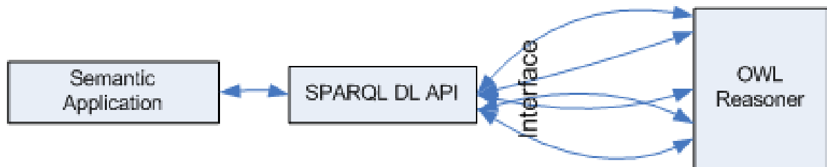
Figure 6.1: The integration of the SPARQL DL API between reasoners and application programs.
